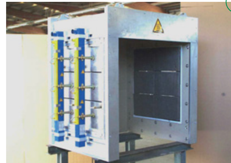
Heating channel with GoGaS metal fiber burners
