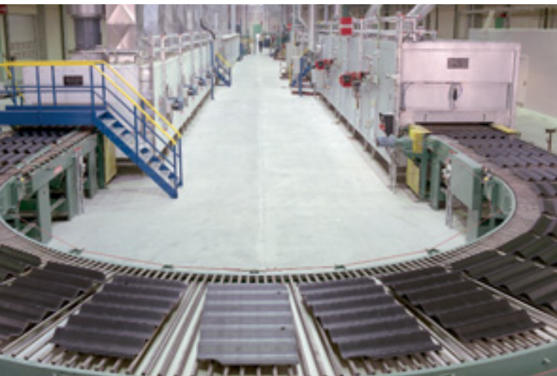
Coating line for corrugated sheets
